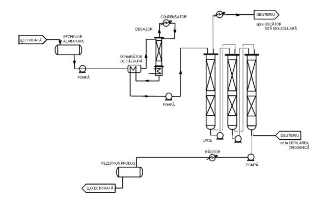
Figure 1.2.2.3.1 Schematic diagram of the isotope exchange system-LPCE
