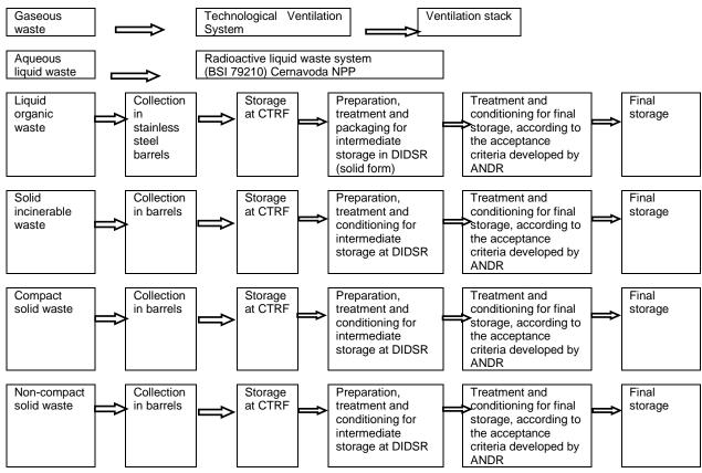
For the management of organic liquid and solid radioactive waste **Temporary storage spaces** will be provided for barrels of radioactive waste resulting from the operation and periodic maintenance of CTRF ready to be transferred for treatment and conditioning according to the control process of radioactive materials Cernavoda NPP [13].
