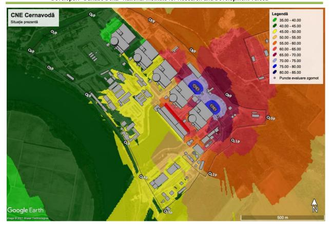
Figure 3.7.1 Noise map for normal operation
