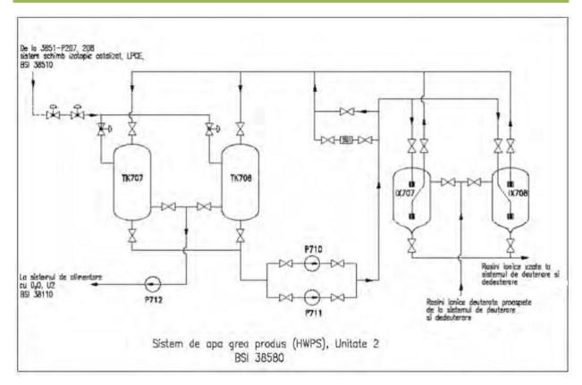
Figure 1.3.1.8 Product heavy water supply system (detritiated heavy water) HWPS - Unit 2
