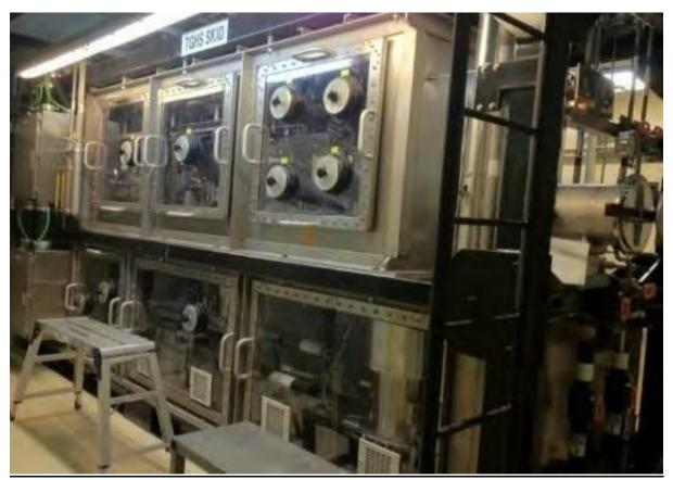
Figure 1.2.2.3.3 WTRF-Korea tritium gas handling and storage system
