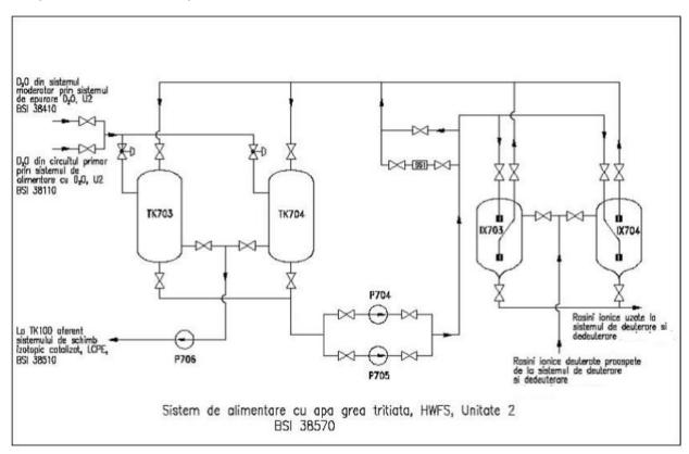
Figure 1.3.1.3 HWFS Tritiated Heavy Water Feed System (Unit 2)
