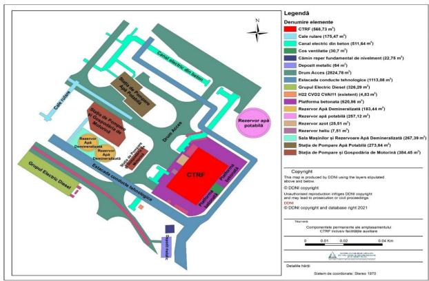
**Figure 1.2.3.4.1** Map of land areas occupied by each of the permanent components of the CTRF project
