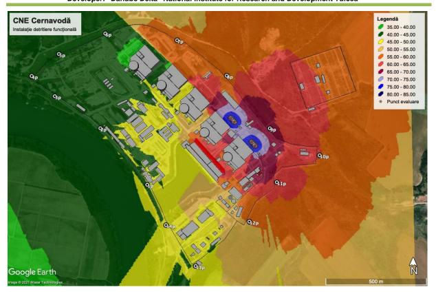
Figure 5.2.6.1 Noise map for CTRF operation
