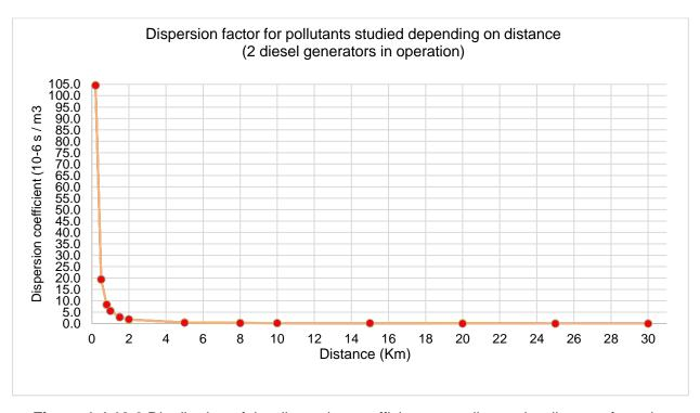
**Figure 1.4.13.2** Distribution of the dispersion coefficient according to the distance from the stack at ground level (2 Diesel generators in operation)
