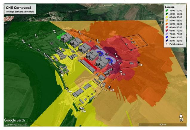
Figure 5.2.6.2 - 3D noise map for CTRF operation
