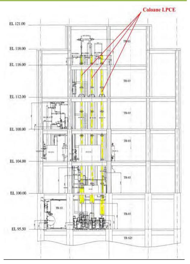
Figure 1.3.1.4 Catalytic isotopic exchange columns. Vertical section through the CTRF building
