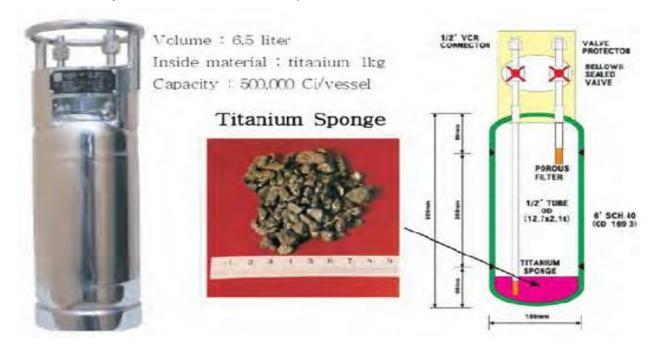
**Figure 1.3.1.6**Container model for storing tritium on a titanium bed at WTRF-Korea Source: "Nuclearelectrica" SA National Society, Presentation Memorandum - Construction works for Heavy Water Tritium Removal Facility, Variant for authorities - May 2019
