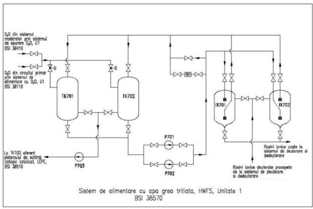
Figure 1.3.1.2 HWFS Tritiated Heavy Water Feed System (Unit 1)
