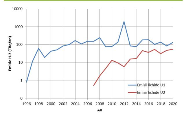
Figure 4.7.1.1 Annual emissions of tritium in the form of liquid effluents from Cernavodă NPP
