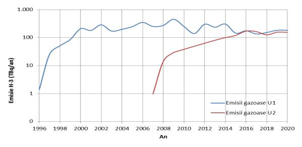
Figure 4.7.1.2 Annual tritium emissions in the form of gaseous effluents from Cernavodă NPP
