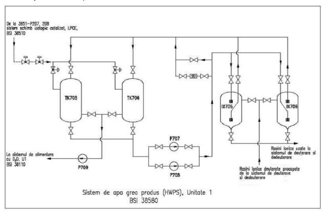
Figure 1.3.1.7 Product heavy water supply system (detritiated heavy water) HWPS - Unit 1
