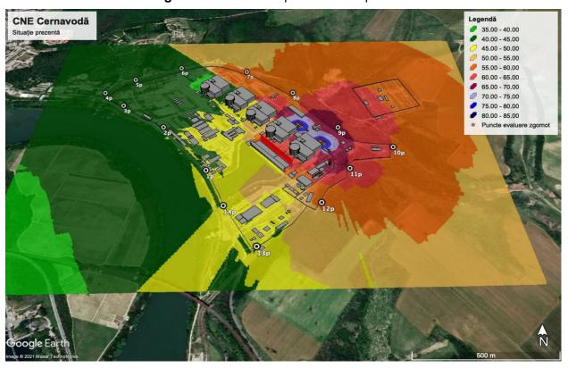
Figure 3.7.2 - 3D noise map for normal operation
