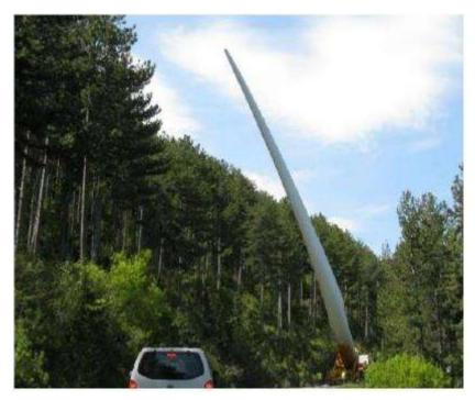
Figure 2-12: Transporting blades using a bladelifter vehicle.
