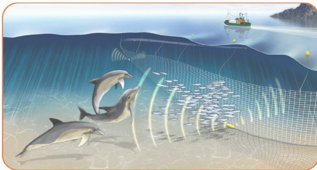
Illustration of how a pinger works. Image designed for the Cornwall Wildlife Trust by Andy McLaughlin at www.tcistudio.co.uk
