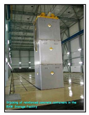
FIGURE 2.2-4 REINFORCED CONCRETE CONTAINERS FOR DISPOSAL OF RAW IN NDF
